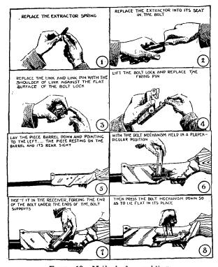
FIGURE 18.—Method of assembling.
