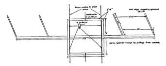
FIGURE 52.—Overhead target carrier.
