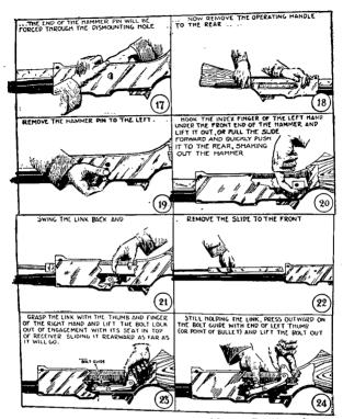
FIGURE 3.--Method of disassembling--Continued.
