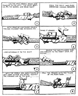
FIGURE 3.—Method of disassembling.
