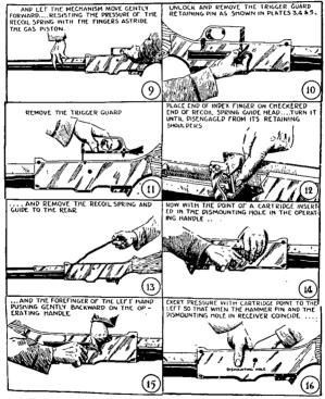
FIGURE 3.—Method of disassembling—Continued.
