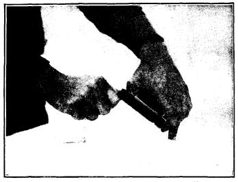
FIGURE 21.—Disassembling magazine, first operation.
