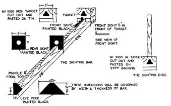
FIGURE 31.—Construction of sighting bar and sighting disk.
