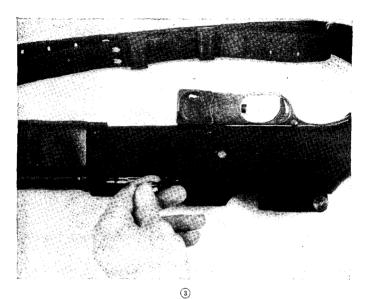
Figure 20.—To remove and replace extractor without disassembling rifle—Continued.
