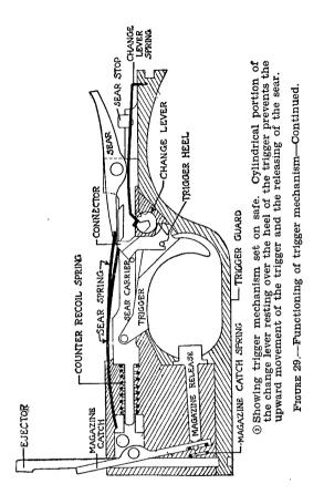
■ 24. Setting Change Lever.—a. Assemble the change lever and spring to the trigger guard. The toe of the change lever is seated in one of the longitudinal slots on the change lever, and as the lever is turned from one position to another it seats in the other slots. The only function of the spring and the longitudinal slots is to hold the change lever in the position in which it is set.
