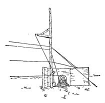
Figure 53.—Rear view of nonoverhead range butts, showing drum, guide wires, and bumper.
