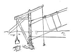
Figure 56.—Rear view of climbing and diving target and method of securing target to frame.
